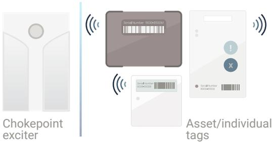
**1. When in close proximity to a chokepoint exciter, the active RFID tags would transmit its location in relation to the exciter.**
